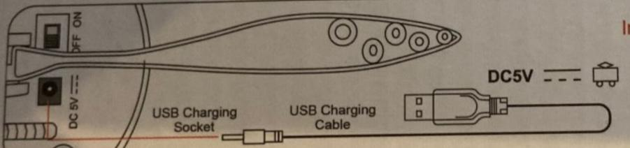
Important note: Please use the original USB cable of this product to connect the transformer with USB socket (such as mobile power supply, notebook computer, desktop computer host, etc.) to supply power to this product The transformer is not delivered.
