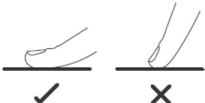
The controls respond to touch, so you don't need to apply any pressure. Use the ball of your finger, not its tip.
