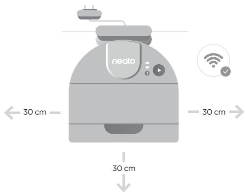
Place the robot against the charge base. When docked properly, the battery icon will light up.
