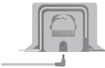
Select a clear area with good Wi-Fi coverage. Make sure the charge base is against the wall and plugged in.
