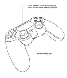
There are several built-in output connection ports in the controller: 3.5mm headset jack, Micro-USB charging port, extension port and built-in speaker. Among them, the 3.5mm stereo headset jack can connect with headset and microphone, allowing Users to receive and transmit audio at the same time.
