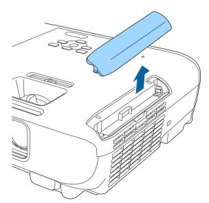
B Pull the air filter out of the projector.
