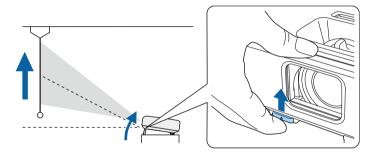
The foot extends from the projector. You can adjust the position up to 12 degrees.
