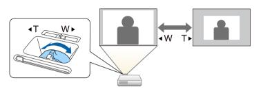
You can correct the focus using the focus ring.
