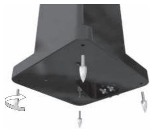
Take the spikes and twist them in a clockwise direction in to the plinths. Ensure they are fully inserted, stand the cabinet up and place it in it's final location. To level, adjust the spikes accordingly, before finally tightening the knurled locking nut to hold the spikes in that position.
