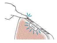
When Envaya is running on battery power, the status and battery indicators will turn off to save power in approximately 8 seconds.
