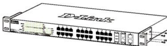
Figure 2.2 – Attach the mounting brackets to the Switch
