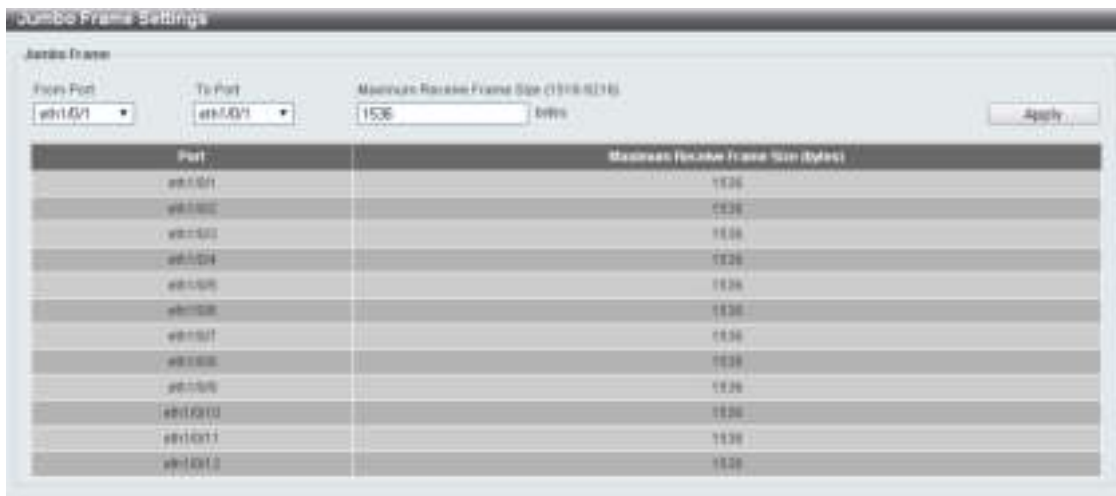
Figure 4.31 –System > Port Configuration > Jumbo Frame
