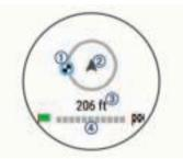
The destination indicator ① shows the direction of your destination relative to the direction you are moving ②. When the destination indicator appears at the top of the circle, you are heading toward your destination. The remaining distance to your destination ③ appears below the circle. The progress bar ④ shows your progress toward your destination.
