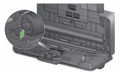
6. Re-install the pre-separation pad by aligning the slots with the holes on the pre-separation pad and snapping it into place.
