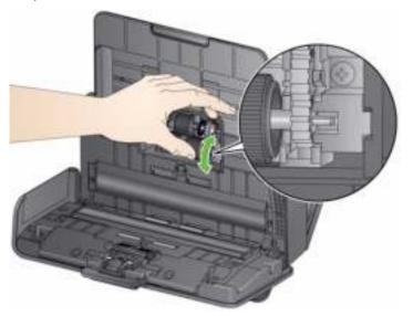
then lift the roller out of position.
