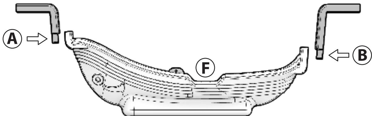
**NOTE:** The plastic parts are labeled, locate and match letters. Short piece fits tall side of boat, long piece fits low side of boat.
