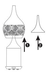
Remove the glass cover and empty the water tank carefully, avoiding the air outlet. Wipe it with a soft, damp cloth to remove any remaining oil from the water tank.
