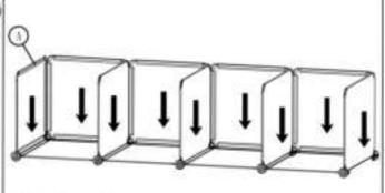
Install panels Insert side panel and back panel according to arrow direction
