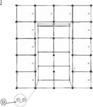
Repeat previous assemble way to spread the cubes until all cubes are assembled.
