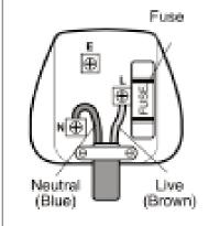
If the mains plug needs to be replaced, proceed as follows: Fuse 5A
