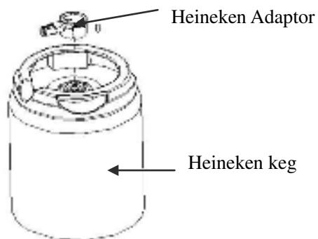
Note: Please take out the Heineken adaptor with collect ways, Press it according the arrow indication, or will damage the fastener
