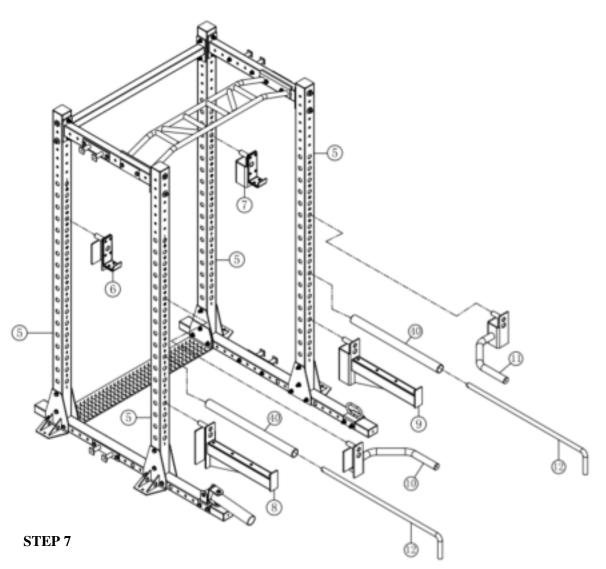
HOOKS, PARALLEL BARS, AND SAFETY TUBES ATTACHMENT.
