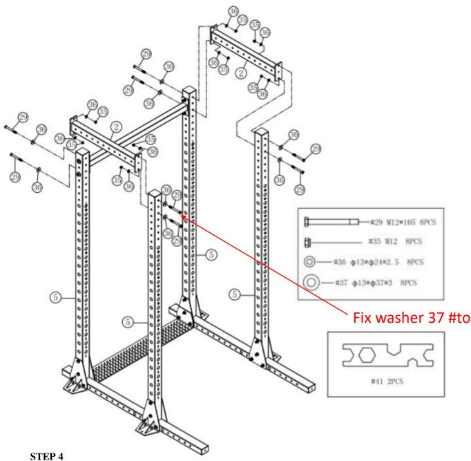
**UPPER CROSS BARS INSTALLATION** Refer to the illustration above for location, and orientation of components.
