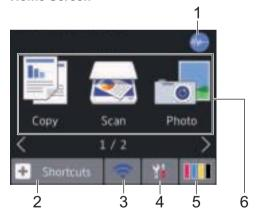
This screen shows the machine's status when the machine is idle. When displayed, it indicates that your machine is ready for the next command.
