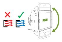
**IMPORTANT:** DO NOT DIRECT HEATED AIR FROM THE VENT ONTO THE VENT MOUNT WHILE IT IS ATTACHED TO THE VENT—this can damage the vent mount and a docked device. When running the vehicle's heater, completely close the vent the vent mount is attached to, or direct the heated air out of the vehicle's lower vents and entirely away from the upper vents.
