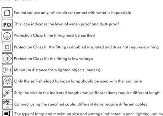
Man a 12 mm Sept 1 Shan hill The type of lamp and maximum size and wattage indicated in each lighting unit must not be exceed; different items require different kind of light sources with different bulb icons
