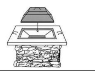
Put the Spark Safeguard Screen onto the top opening of the Fire Pit Body and make sure it sits into it evenly. The Firepit is ready for use.
