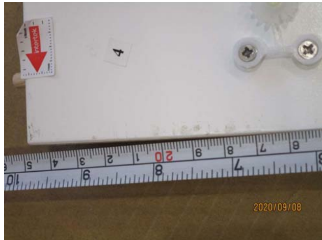
00 defect-minor-dirty mark(3-8cm) on unit (2)
