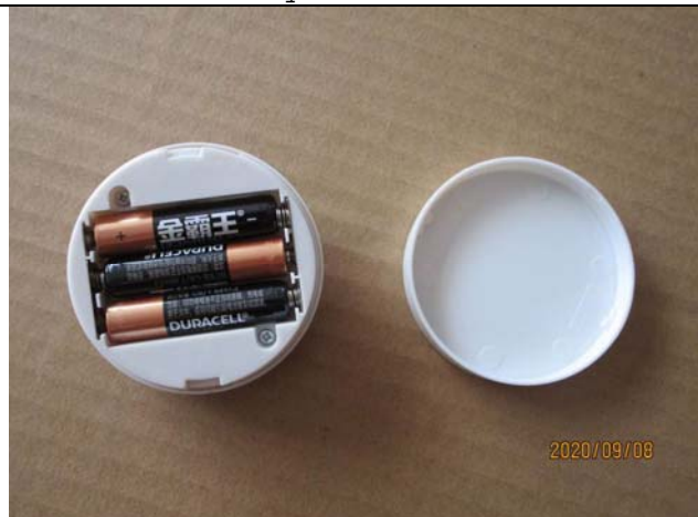
28 battery compartment fitting check (2)
