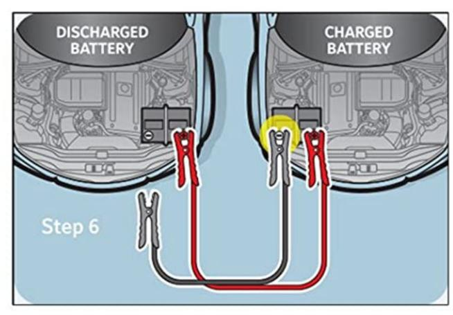
Connect one black clamp to the negative(-) terminal of the charged battery
