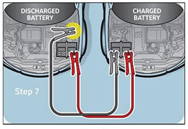
Connect another black clamp to the frame bumper or engine block of the dead battery
