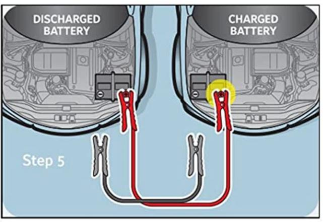
Connect another red clamp to the positive terminal of the charged battery
