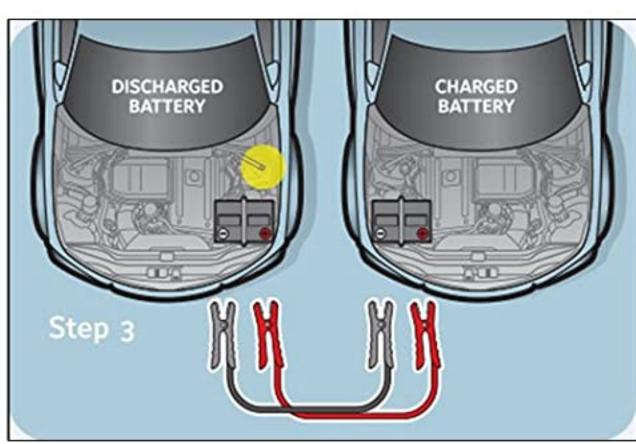
Identify the frame bumper or engine block of the dead battery
