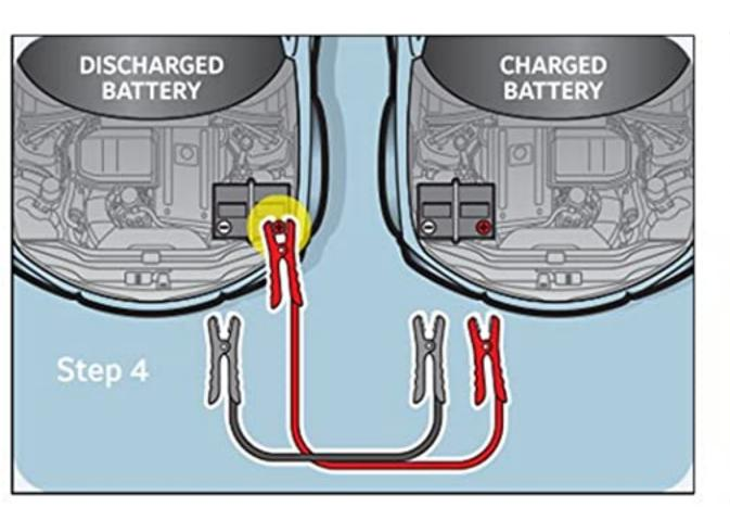
Connect one red clamp to the positive(+) terminal of the dead battery
