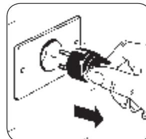
3. Use a cross screwdriver (not supplied with the product) to remove the screws. Remove the air filter, clean it with a detergent (do not use petrol, alcohol, diesel or other similar products) and dry it.
