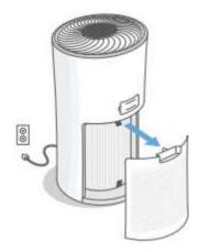
Remove the old air filter and properly dispose of it.
