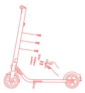
3. Install the external battery on the rail and fix it with the M4 (20mm) 4. Verify that your KickScooter powers on and off. screws (2 pcs) and M3 screw (1 pcs), provided with this product. After they are properly installed, block the screw holes with the rubber stopper.
