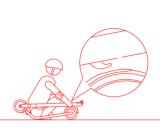
Then fold the handlebar down until it locks into the rear fender.
