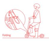
Step on the folding pedal while pushing the handlebar forward slightly.
