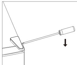
2. Unscrew the top hinge with a philips screw driver.
