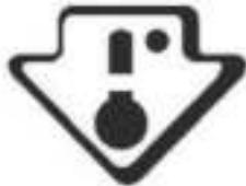
The symbol indicates the location of the coldest part of your refrigerator. This area is in between the vegetable drawer at the bottom and the symbol at the top, or the shelf at the same height. In order to maintain the temperature in this area, make sure not to change the position of this shelf.
