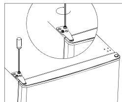
14. Clamp in the hinge cover and hole cover on the top of unit.
