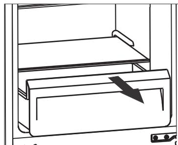
The cover of the vegetable drawer can be removed for cleaning.
