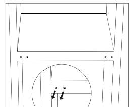
7. Lie down the rear of cabinet on a soft pad. And unscrew the bottom hinge and leveling foot.
