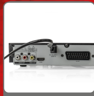
3 ways to connect: HDMI 1.3, Scart or composite (RCA audio/video)
