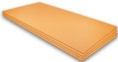
The IS074 increases the efficiency and response time of the underfloor heating foil. These properties result in lower energy consumption. The ISO-74 can only be installed on a flat subfloor. Tape the corners with tape to prevent slipping. Leave approx. 30 mm space for the supply wires. Make sure that the floor is clean and that no sharp objects can get in contact with or fall on the heating foil during installation.
