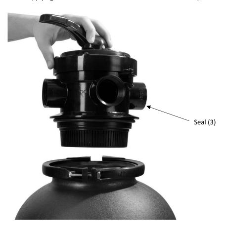
b) Place the valve on the tank. Install the flange clamp around the tank and the valve flange. Tighten the valve just enough to allow it to rotate on the tank for final installation.
