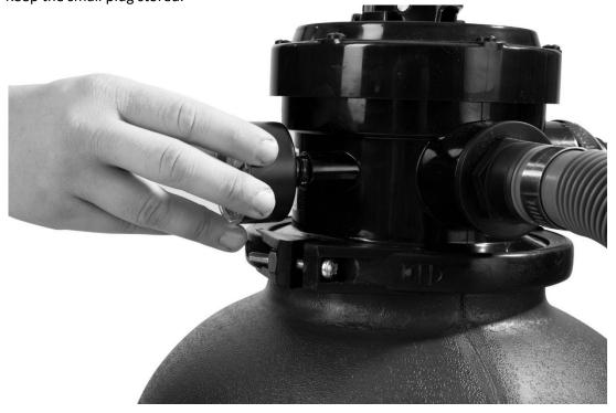
10.) Screw the plug (with seal) into the "WASTE" connection (backwash connection). Remove during backwashing.
