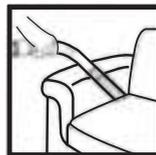
The crevice nozzle is designed for cleaning cracks and corners.
