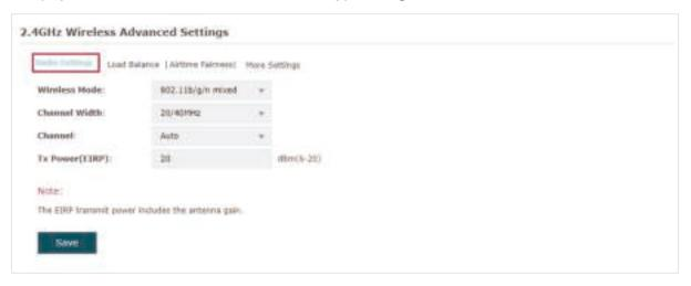
Select the frequency band (2.4GHz/5GHz) and configure the following parameters.
