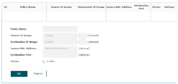
2. Configure the following parameters. When all the configured conditions are met, the client can access the network without authentication.
