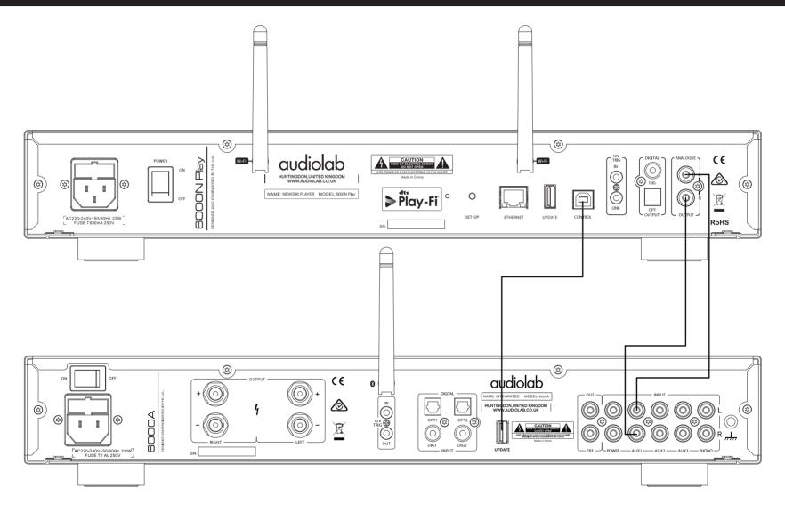
**Note:** 1. For Audiolab 6000N the COAX and OPT outputs transfer the PCM digital signal at up to 24 bit/192kHz resolution.
