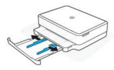
3. Insert a stack of full-size or photo paper into the middle of the paper tray with the short edge oriented towards the printer. For photo paper, make sure the side to be printed on is facing down. Then slide the stack of paper in until it stops.
