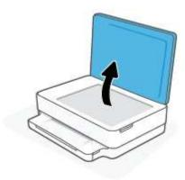
Clean the scanner glass and lid backing by using a soft, lint-free cloth that has been sprayed with a mild glass cleaner.
