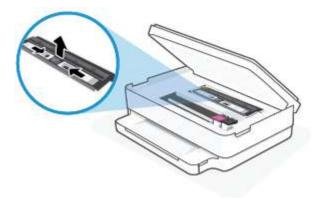
7. If the carriage is in the center of the printer, slide it to the right, and then remove any paper or objects blocking the carriage path.
