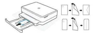
**4.** Slide the paper-width guides to the left and right edges of the stack of envelopes until they stop at both edges.
