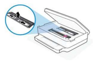
**c.** Lift the duplexer cover up and remove jammed paper.
