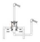
3) After the test is completed, plug all the pipe outlets with a plastic stopper and open the faucet.
