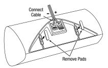
4. Use the supplied screws to attach the speaker to the wall-mount bracket. The screws thread into the center foot-rest openings that were exposed when you removed the rubber pads in the previous step.
