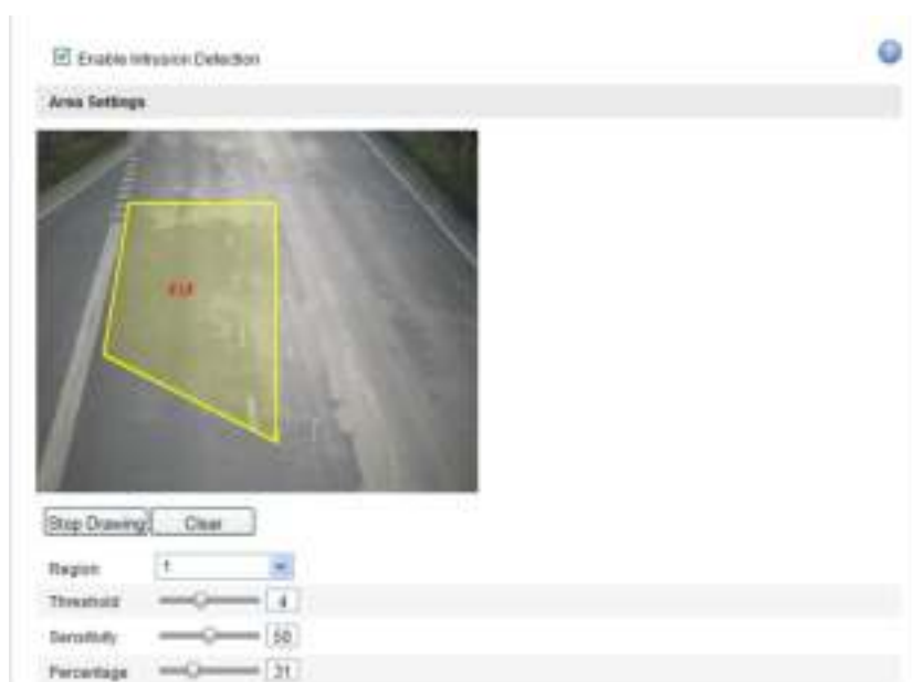
Figure 6-63 Configuring Intrusion Area
