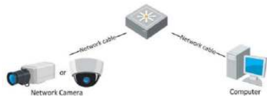
Figure 2-2 Connecting via a Switch or a Router
