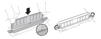
Using firm, even pressure, push DIMM into socket until clips snap into place. Do not assist clips.
