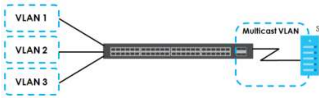
Figure 144 MVR Network Example
