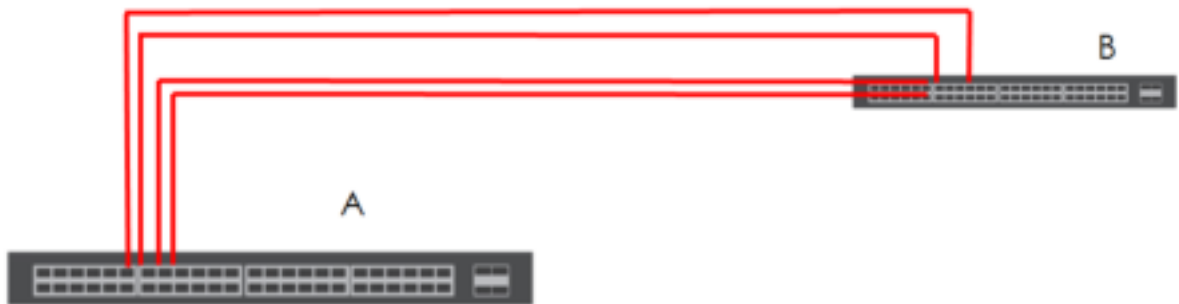
Figure 125 Trunking Example - Physical Connections
