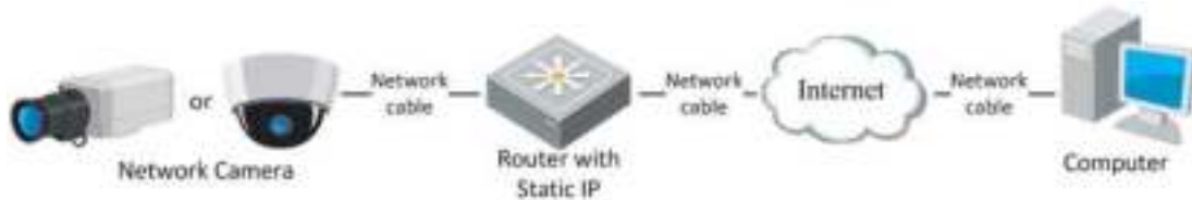
Figure 2-4 Accessing the Camera through Router with Static IP
