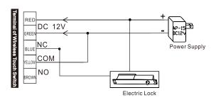
Wireless touch switch connect with electric lock
