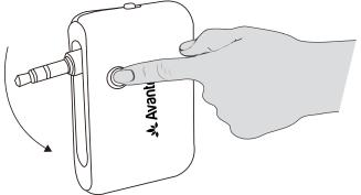
**Step 2** Plug the Avantree Bluetooth CK210 into the 3.5mm port of car stereo then turn CK210 ON.
