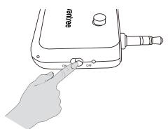
**Step 2** Press and hold the MFB for 3 seconds to enter pairing mode(Note: On first use the CK210 will automatically enter pairing mode).
