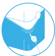
Optional fabric pre-filter. A fabric pre-filter captures larger particles and increases the lifetime of the main filter.
