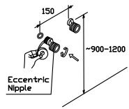
**Step 1** As shown, install the accessories and attach the tape.
