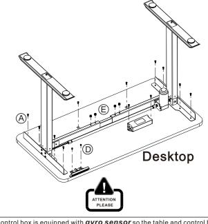
Control box is equipped with *gyro sensor* so the table and control box must be leveled and screwed into tabletop in order to work properly or else it will not move up and down.
