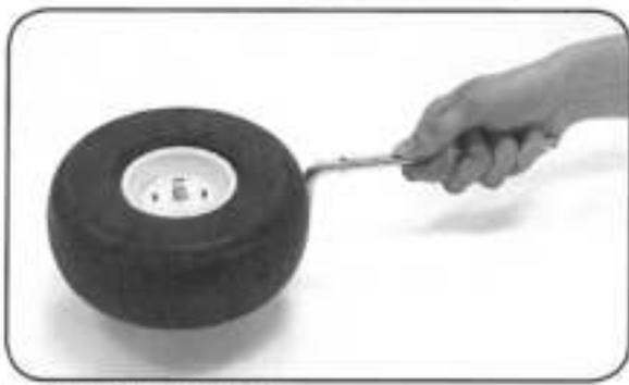
Slide wheel then hubcap onto axle.
