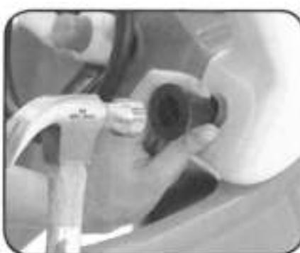
**Place axle cap tool over ignition base and hammer.**
