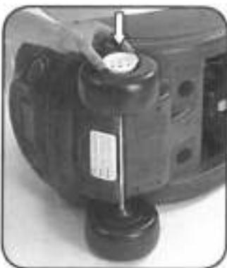
**Hold in place and hammer top hat onto axle.**
