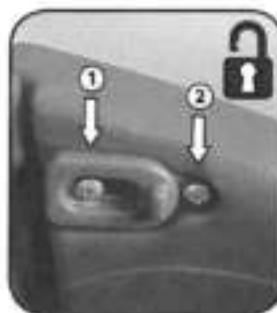
Latch in permanent "locked" position; install (2)  $\frac{1}{2}''$  (1,27) screw.
