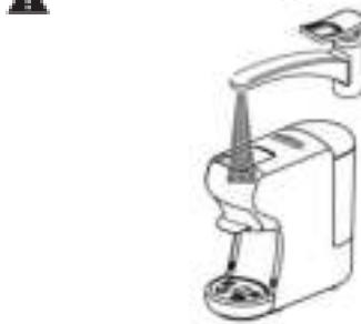
**⚠ Do not use the appliance if the water tank is empty. Make sure the water tank is filled at least to the "MIN" marking.**
