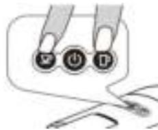
Press the small and large cup buttons simultaneously to start the internal rinsing cycle.
