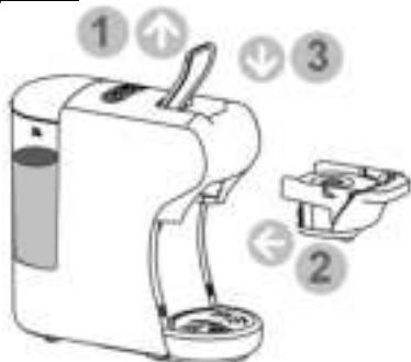
Lift the lever and insert an empty adapter (without capsules or coffee). Lower the lever to close. Place a large cup (min. 250 ml) on the removable grid.
