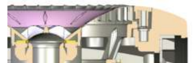
Figure 39 Cross section of complete Uni-Q driver and trim ring
