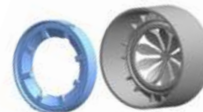
Figure 12 Modified surround support and tangerine waveguide viewed from the rear to show added ribs
