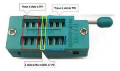
The test positions TP1,TP2,TP3 are used to test diodes, capacitors, resistors, transistors, fets, etc..
