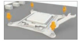
**Installation of the mounting brackets** Attach the two Intel mounting brackets (4) to the underside of the CPU cooler using the M3x3 screws (11).
