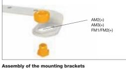
Attach the two short AMD mounting brackets (5) to the underside of the CPU cooler using the M3x3 screws (11).
