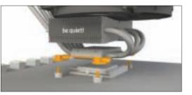
and affix by turning the AMD M3x15 (10) from the rear side of the motherboard.
