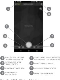
Note: The 360fly 4K's AutoPilot feature sets your application to automatically pan your image to the area of footage that has the highest degree of motion. To use this feature within your camera's live-view, just tap the AutoPilot icon . Use the slider located on the left of your display to adjust the sensitivity level.
